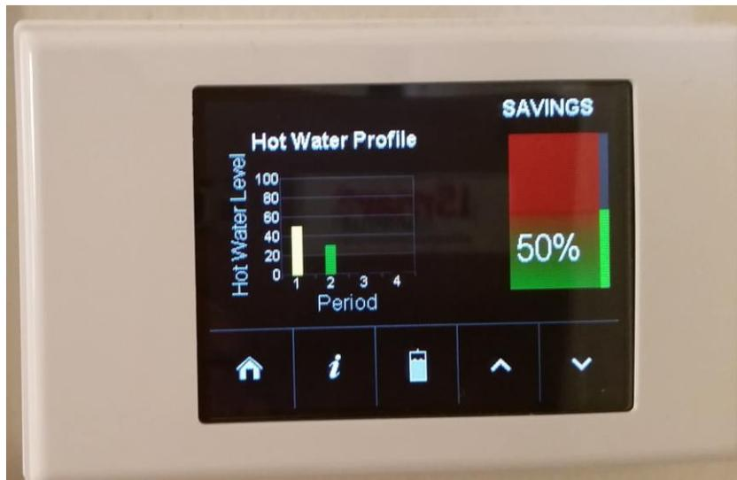
The system is comprised of a controller and LCD user interface, both housed in a small box mounted on or near the cylinder, along with two temperature sensors. You'll need an electrician to retrofit the iSmart to your cylinder's power supply and install the sensors.
